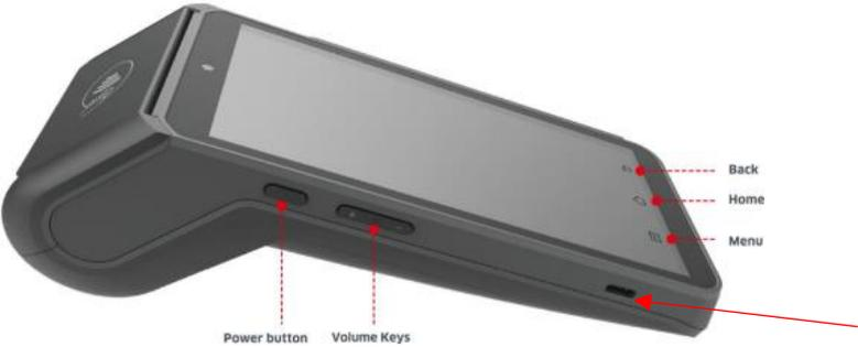
The diagram shows the terminal from a three-quarter perspective. On the left side, there are three physical keys: a Power button and two Volume Keys. On the right side, there are three virtual keys: Back, Home, and Menu. At the bottom of the screen, there are three virtual keys: Menu, Home, and Back. At the bottom of the terminal, there is a USB TYPE C Charging port.
